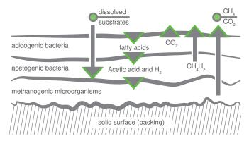
The microorganisms are fixed on the carrier material and thus make it possible to decouple the generation time from the residence time of the substrates. Optimal properties of the carrier material promote the settlement of syntrophic communities.
